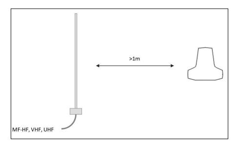
1.1.4 The antenna unit should be installed with a 360° clear view of the sky. However, minor obstructions such as a mast will not degrade the antenna performance severely, if a separation distance larger than 15 times the diameter of the obstruction is kept.
